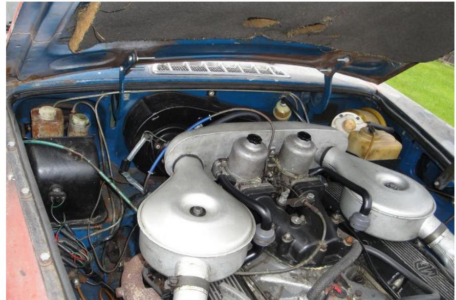
Some parts in the engine bay appeared to include new air cleaner units and claws over the exhaust manifolds. The car shows signs of lengthy storage and corrosion possibly from occasionally damp conditions. Underneath a telescopic rear shock absorber modification has been fitted. At some stage.
