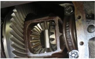
Back axle surprise Peter Nixon is restoring an MGB Roadster with a V8 conversion and on checking a second hand V8 back axle before installation he was surprised by what he found. He noticed a broken piece of a bronze thrust washer from the planet gears lying in the oil - not what one wants to see. Using a screwdriver he could move the planet gears by about a millimetre on the pinion shaft, so obviously this called for new thrust washers to be fitted. As the remains of the planet gear thrust
