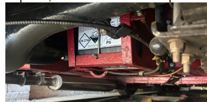
Peter Cope's twin 12-volt conversion, with revised bar & clamp orientation.
