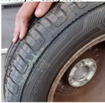
Peter Berry reports "a good friend of mine recently had his RV8 fail the MoT test on account of the front offside tyre being worn down to the cords from a cut into the side wall. It seems that an exhaust bracket had been fouling the inside wall with the steering wheel on a right-hand lock. A blowout could have been quite imminent with disastrous consequences had this not been picked
