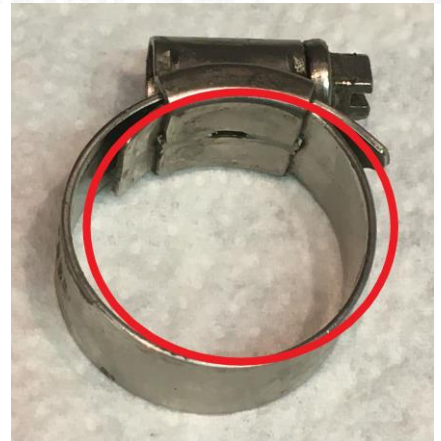
Worm drive clip showing distortion if the wrong size is used
