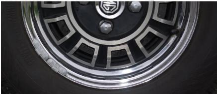
corroded Dunlop composite wheel is a skilled process which involves splitting the rim from the alloy centre, removing corrosion, rechroming the steel rims, refurbishing the alloy centres and then reassembling and balancing the wheel. Typical cost is around £600 a wheel including VAT. If the wheel has been restored before it will need a careful inspection to assess if the wheel could be restored again. Renowheel in Wales offer this full service.
