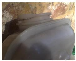
RV8 cooling problem traced to a small crack in the neck of the expansion tank
