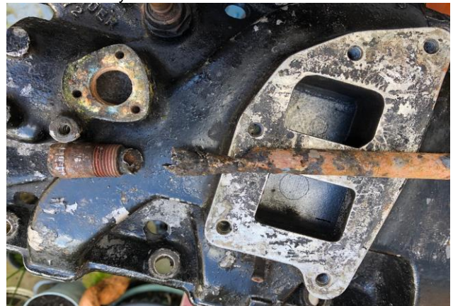
Severely corroded internal Heater Feed Pipe 90611532. (Ralph Hardwick)
