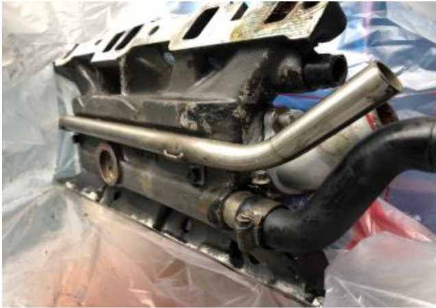
Stainless steel replacement Bypass Pipe Heater Outlet 603049 attached to the underside of the intake manifold (Ralph Hardwick)
