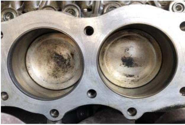
Removing the heads discovered that one of the liners was slightly lower than the block deck height - a slipped liner (Ralph Hardwick)
