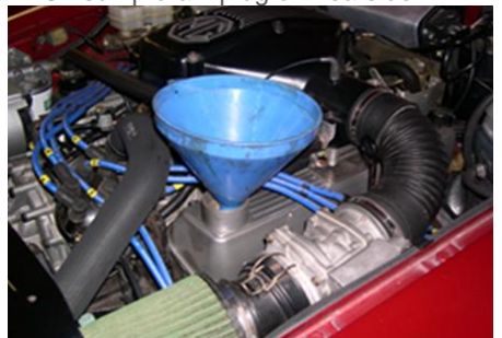
RV8 - oil fill point and funnel.
