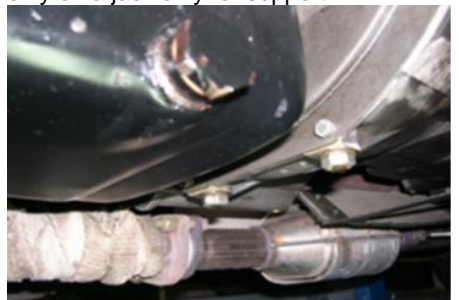
RV8 - sump drain plug on nearside
