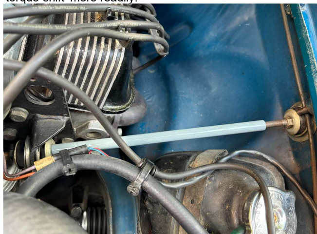
Stabilizer Bar reinstalled on no. 201, problem solved.
