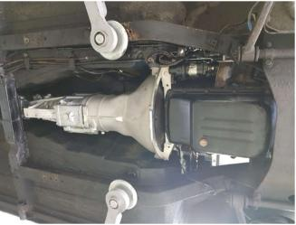
The slave cylinder is mounted within the gearbox, which makes it more difficult to get to, should any maintenance be required but modern components such as this are a lot more reliable these days and I shall worry about the consequences, should the need ever arise. If the 'box ever has to be removed, engine removal is no longer required to split it from the gearbox.
