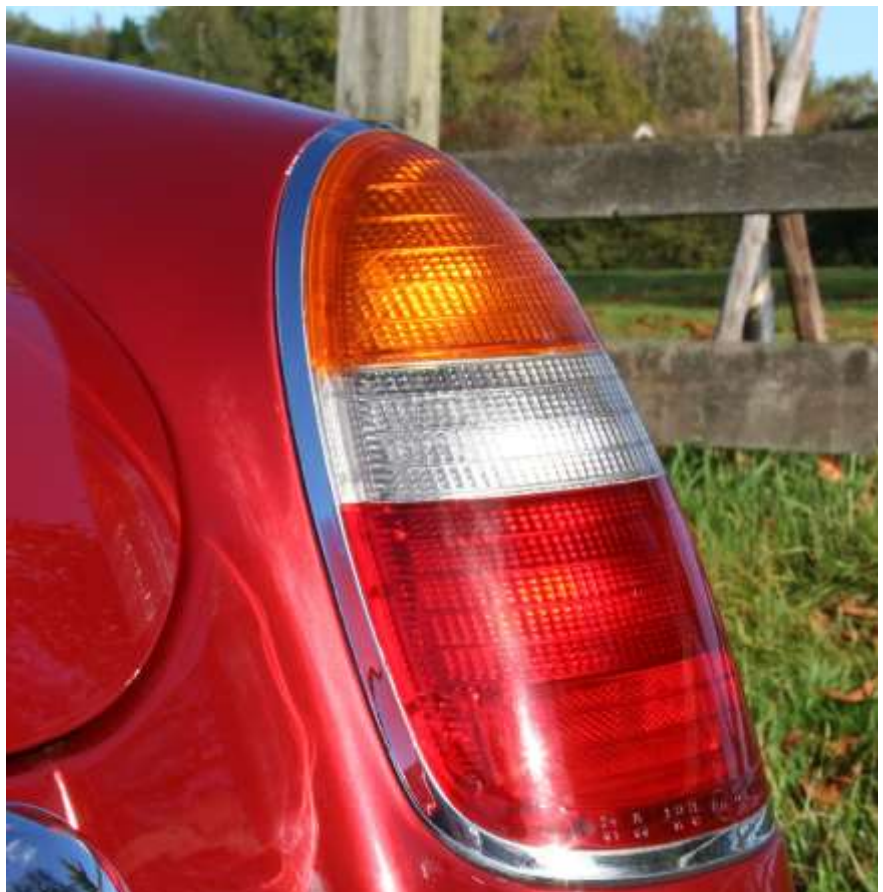
All three lenses and the back of the rear lamp are in one unit although the parts are individually made and assembled as a single unit
