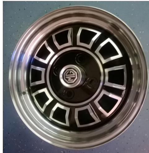
New all-alloy replacement 15" V8 lookalike wheel with a polished rim supplied by Clive Wheatley.
