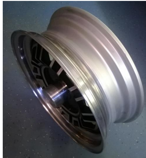
New all-alloy replacement 15" V8 lookalike wheel with a polished rim supplied by Clive Wheatley.
