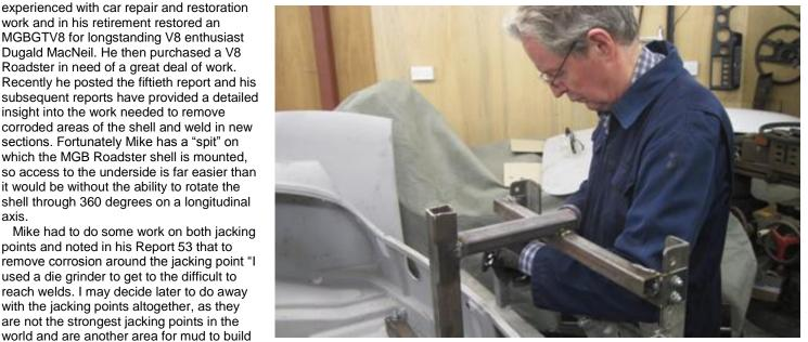
Mike had to do some work on both jacking points and noted in his Report 53 that to remove corrosion around the jacking point "I used a die grinder to get to the difficult to reach welds. I may decide later to do away with the jacking points altogether, as they are not the strongest jacking points in the world and are another area for mud to build
