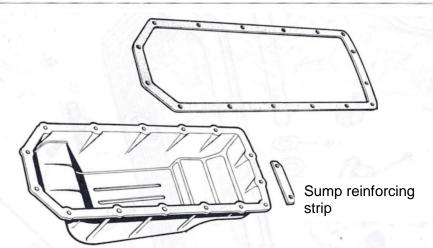
Modification to reduce MGV8 sump gasket leakage
