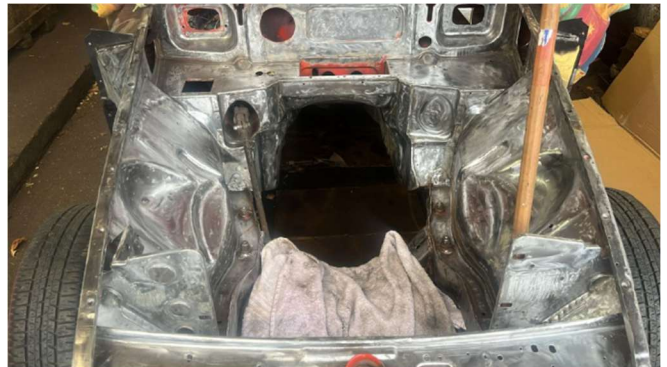
The usual areas up under the front wings had seen better days when the wings were removed, so these were cut out and repaired as necessary.
