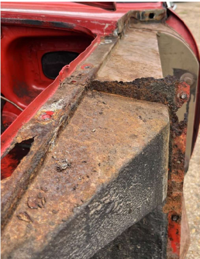
The usual areas up under the front wings had seen better days when the wings were removed, so these were cut out and repaired as necessary.
