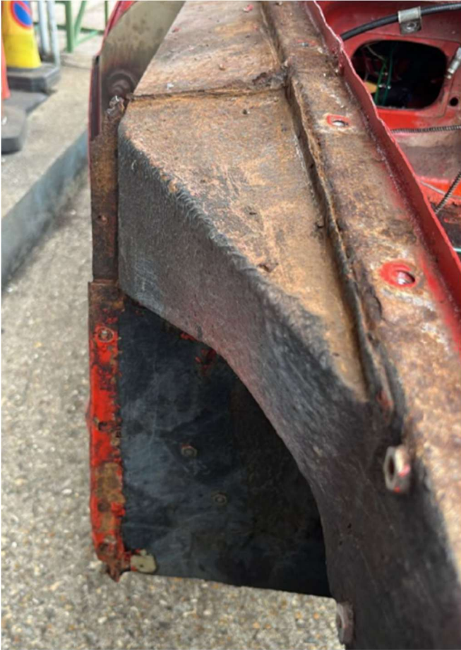
The usual areas up under the front wings had seen better days when the wings were removed, so these were cut out and repaired as necessary.
