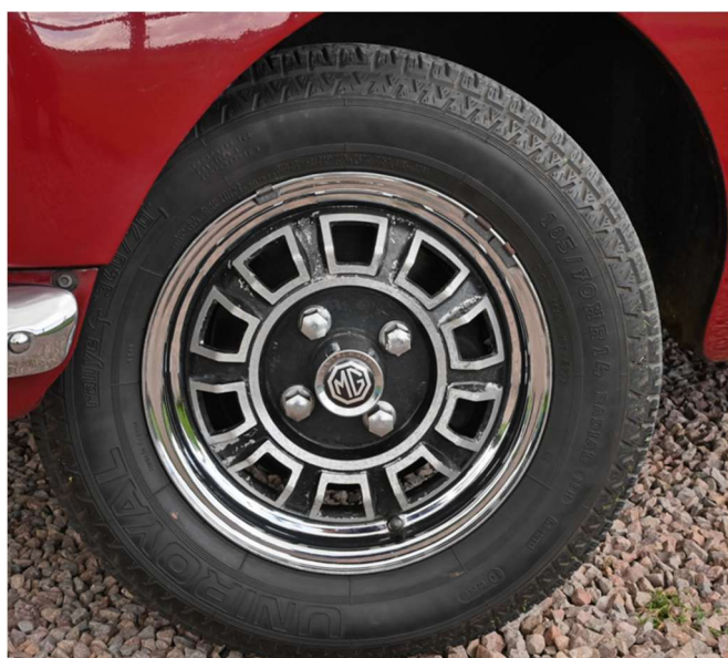
Original Dunlop composite wheel with a chrome rim and alloy centre
