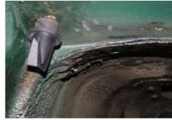
New drain tube is shorter than the original part (see photo above right). Access with the gearbox in place is very restricted and difficult.
