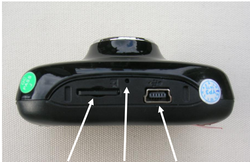
Underside: Memory card slot, Reset hole and USB socket
