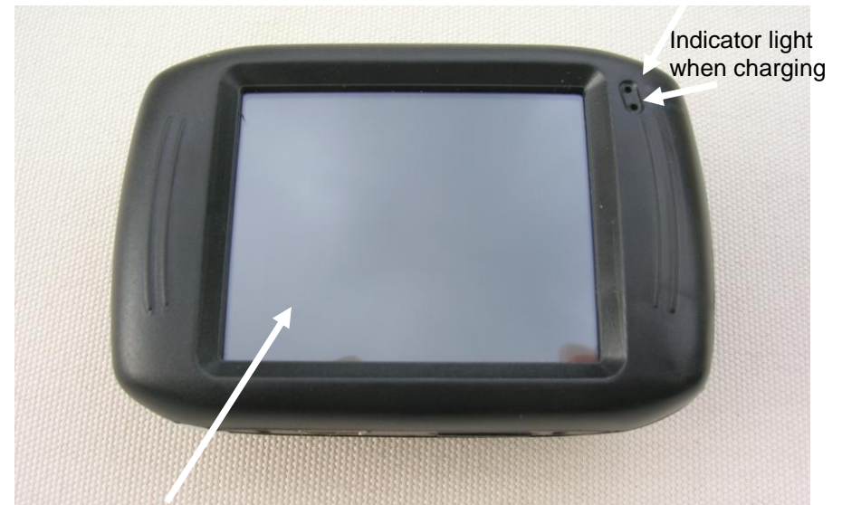
Back: LCD TFT screen (40mm x 30mm). (Front: Lens )
