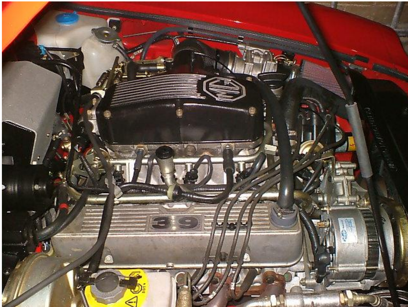
MG RV8 photo profile – Injected 3.9 litre V8 in the engine bay
