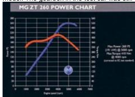
Performance chart show the broad torque curve and the power curve rising to 260PS. (MG Rover)
