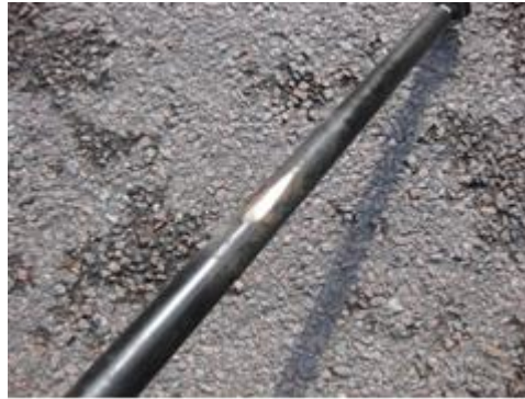
Panhard rod polished from friction contact with the diff casing. (Photo: Angus Munro)
