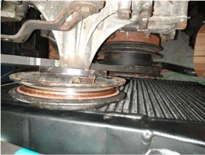
New belt run to the alternator
