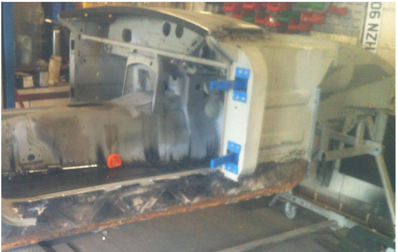
Indication of the extent of the rot in the outer sills , fortunately apart from surface rust on the side member behind the sill there was nothing much to do except bead blast off the rust, paint with acid etch and then weld on the new sills. (2279)
