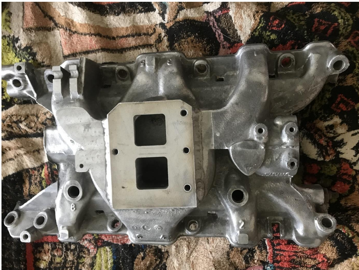
Modified Range Rover inlet manifold , 10mm machined off and 10mm plate welded on to mount the tubular plenum. (1644)
