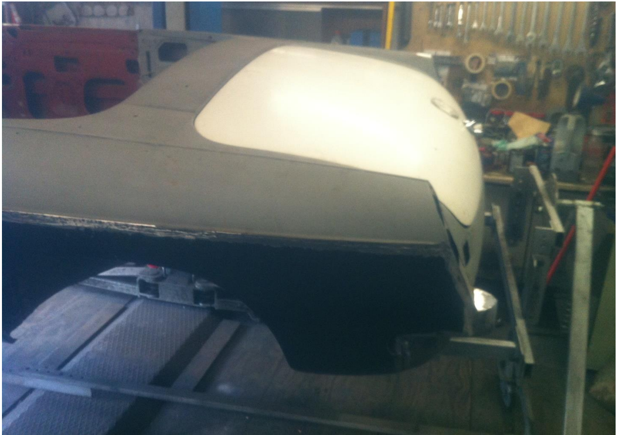
New rear half wing welded into place. (2315)
