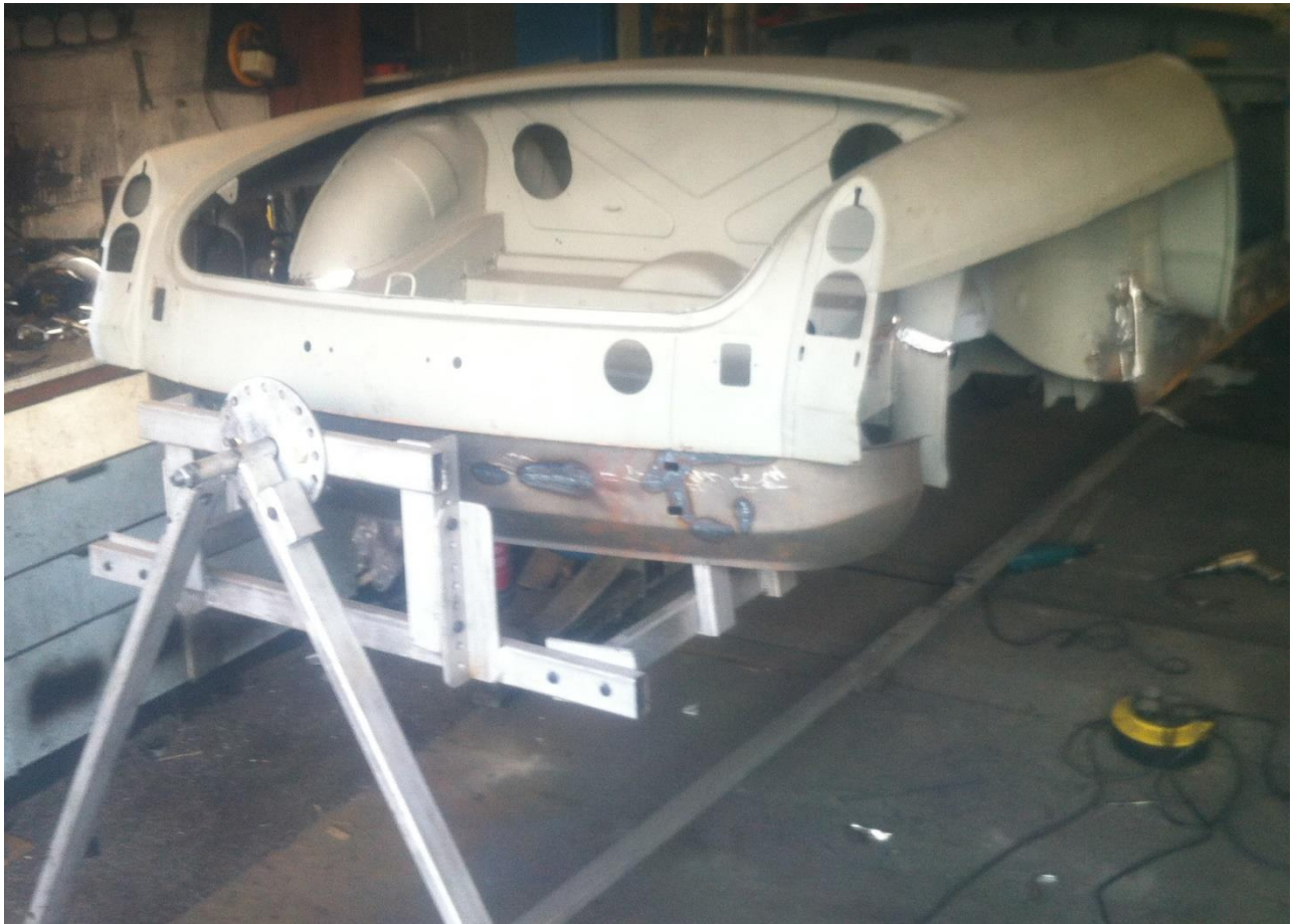
Stripped car body on the rotisserie - the rear wings were cut at the swage line for new rear half wings to be fitted, the joins are hidden behind the chrome strip. (2281)
