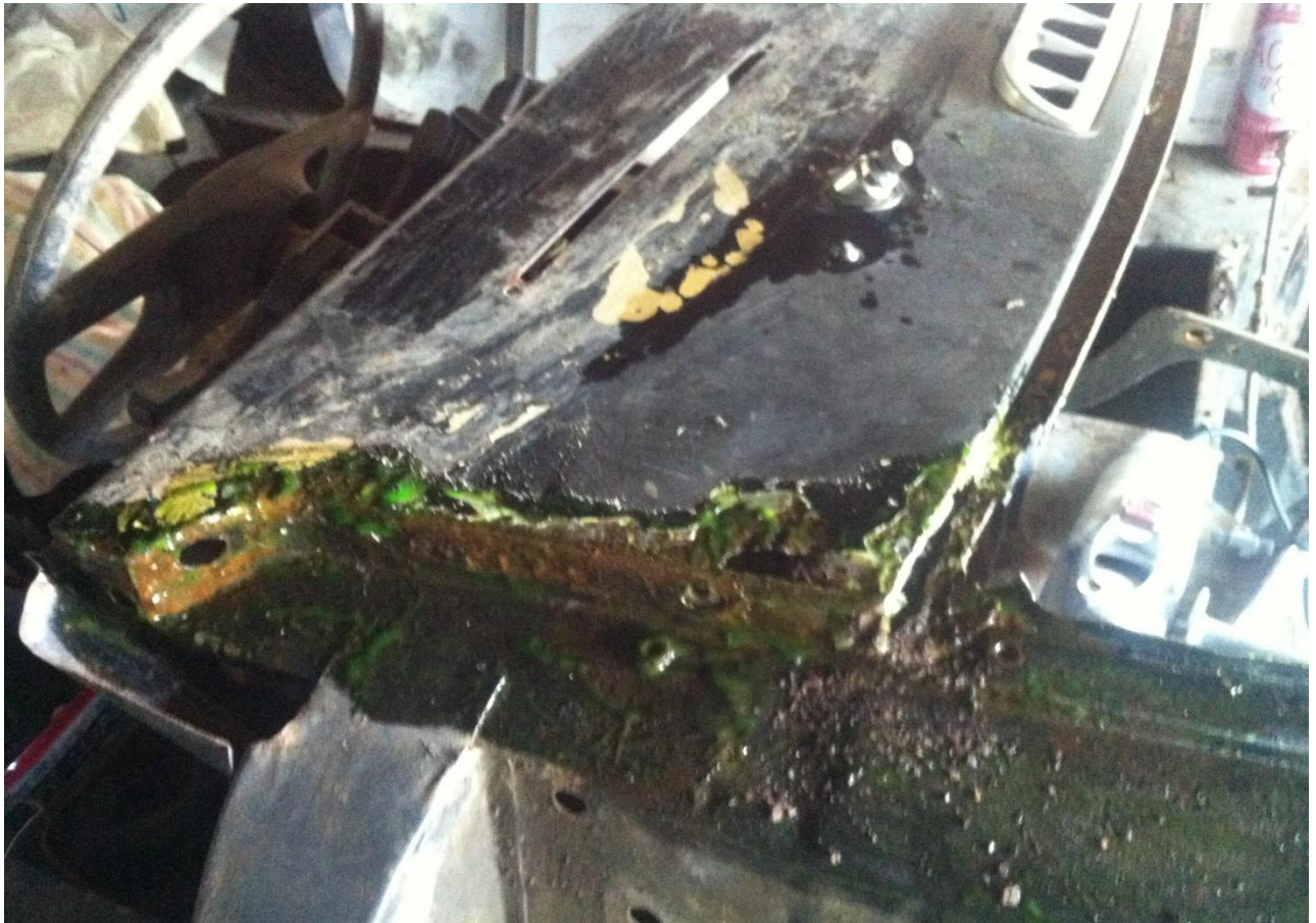
The state of the shroud panel on the rust bucket, the state of the shroud panel was the reason for its replacement with a new panel suitable for new chrome bumper front wings. (1106)
