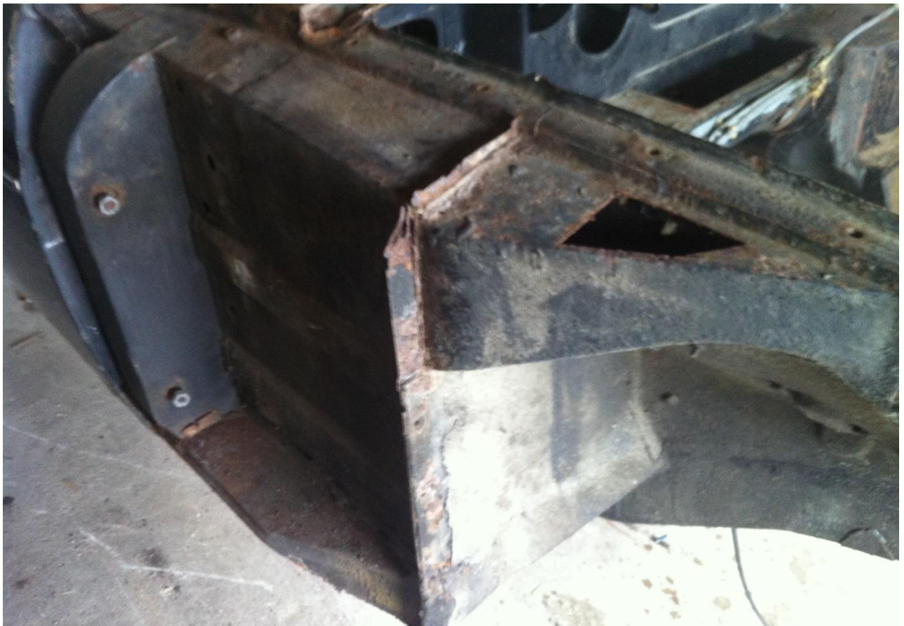
The state of the reinforcement panel behind the front wing on the rust bucket. (1091)
