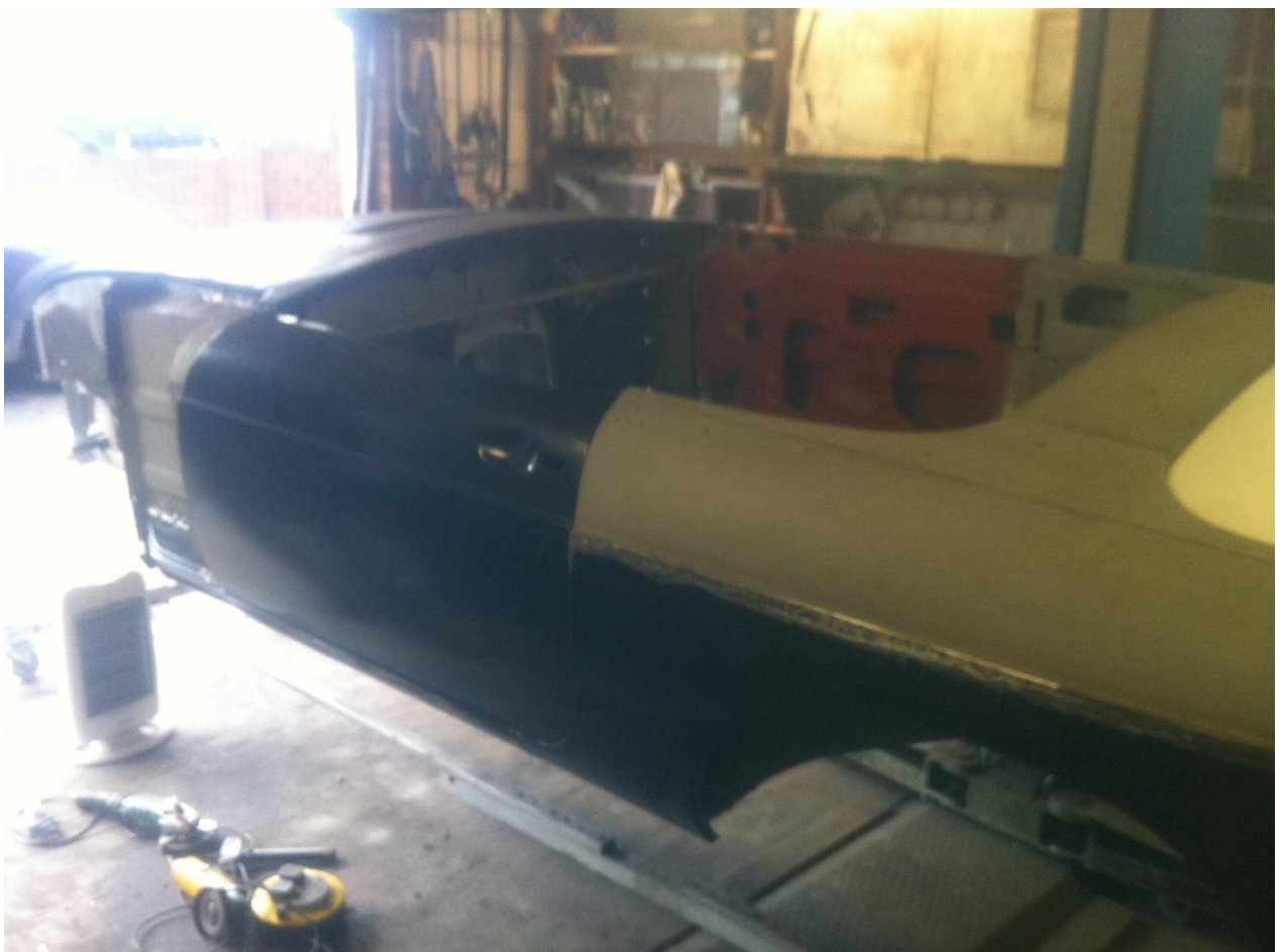
Lining up the new rear half wing and door prior to welding in the wing. (2314)
