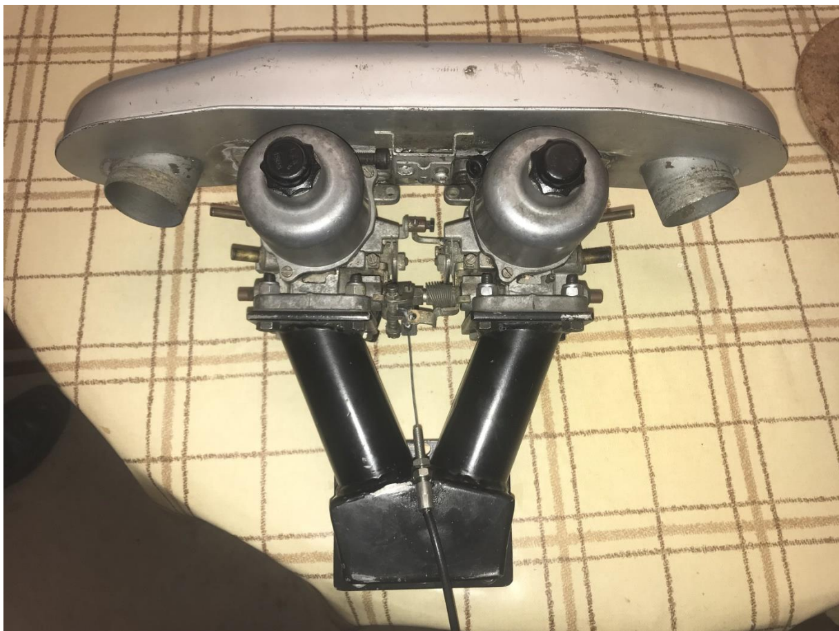
Inlet manifold & plenum with the Rover SD1 carburetors and MGB GT V8 airbox. (2360)
