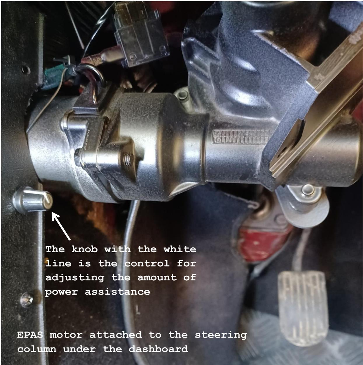
The knob with the white line is the control for adjusting the amount of power assistance
