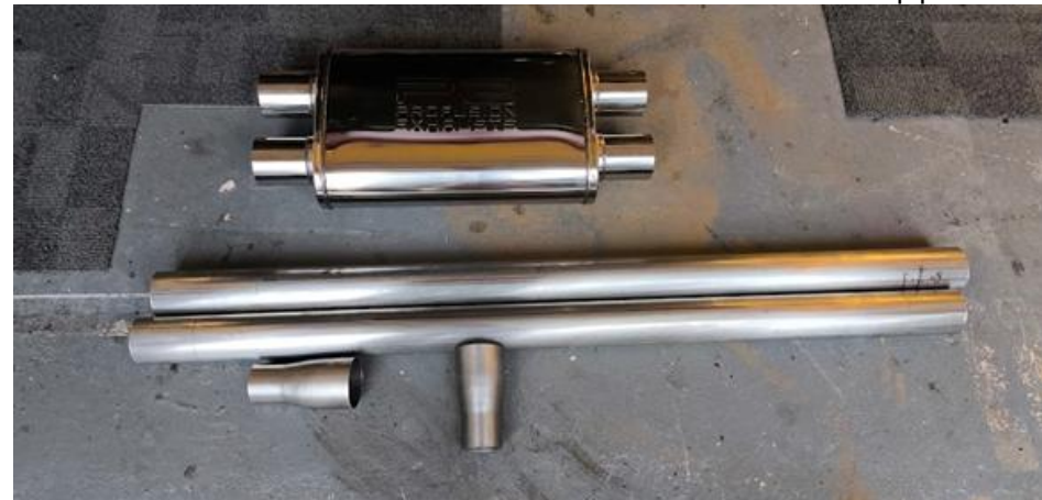
X pipe exhaust box in stainless and stainless 2 1/4" pipes for the exhaust
