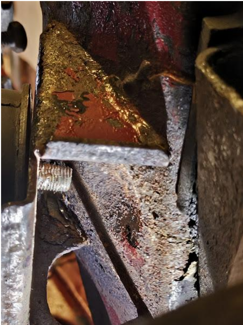
Gear box cross member modified to suit the LT55 and to fit the twin pipes in.
