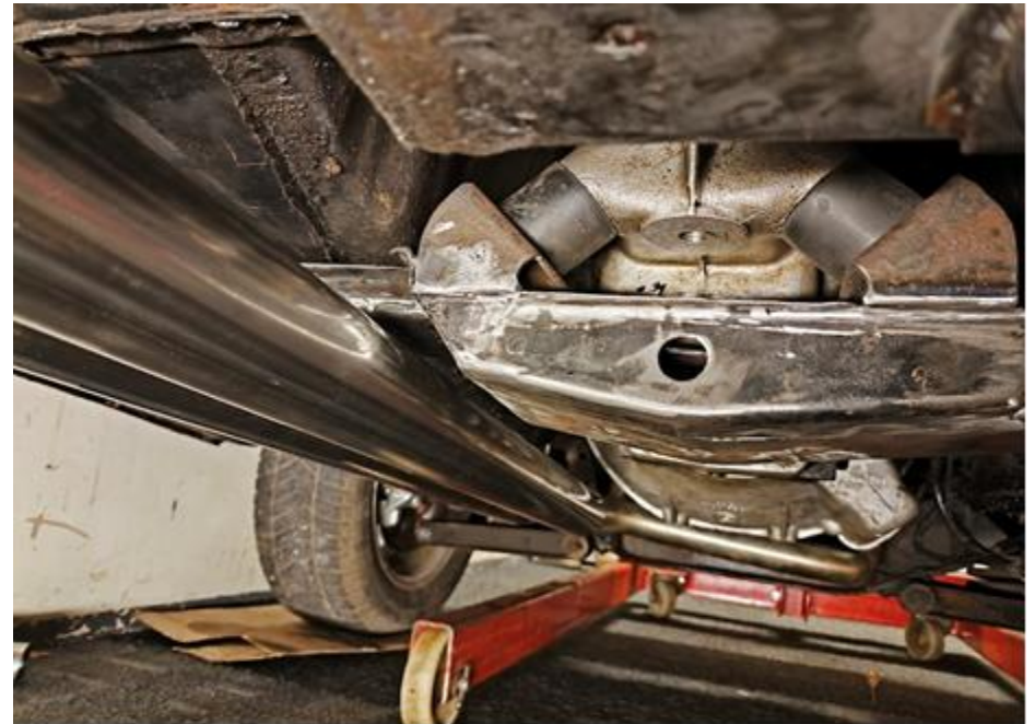
Gear box cross member modified to suit the LT55 and to fit the twin pipes in.
