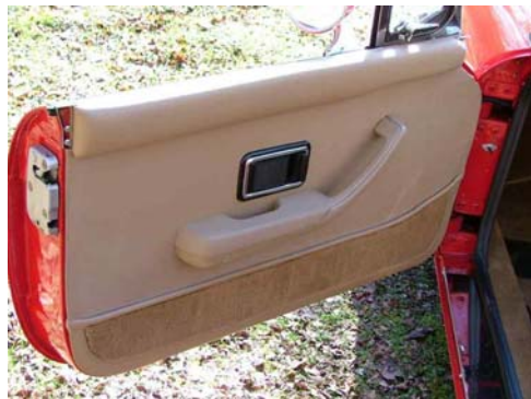
Door panels with the armrest from a Vauxhall sprayed with "Vinylkote" to match the biscuit interior. Note no speakers or
