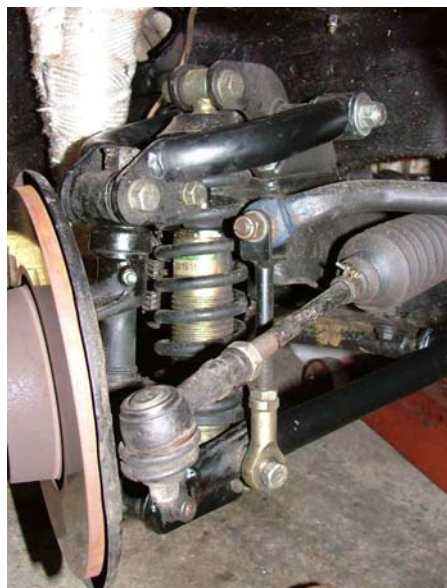
Front suspension with the coilover damper conversion and the lagged RV8 exhaust above and behind the brake disc. (Photo: Geoff King)
