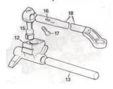
Gearbox selector plate 22B386, later replaced by 22B726, is item 12 in this diagram. Item 18 is the remote control shaft which transmits the gear lever movements to the selector plate when you select gear. (Diagram from page 108-C44 Parts Catalogue AKM0039)
