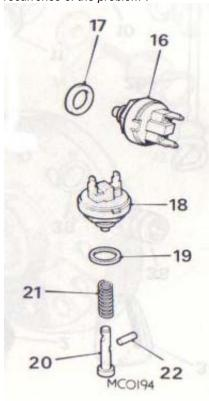
Plunger isolation switch 22B406, later changed to 22B727, is item **20** in this diagram with the overdrive isolation switch (**18**) and reverse light switch (**16**) both part number 13H2154. (Diagram from page 108-C45 Parts Catalogue AKM0039)
