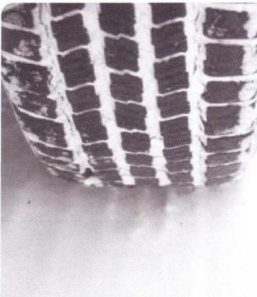
An ice tyre will have sharp edges the treads which are designed to remain open and clear of any surface snow so that a sharp edge is always presented to the hopefully ice, providing grip. Any open tread winter tyre will generate more road noise than a summer tyre and ideally would not be used in the summer, but tyre manufacturers' advice is that winter tyres are perfectly OK for summer use but they will have a higher wear rate.
