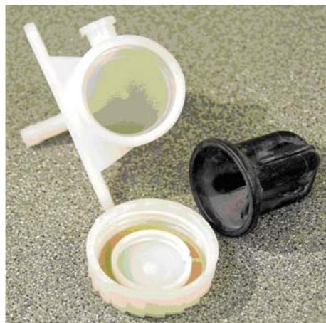
*AP Nylon Master Cylinder reservoir with diaphragm*
