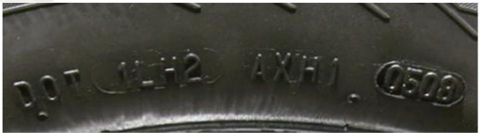
the USA have the DOT code as required by the US Department of Transport (DOT). It specifies the company, factory, mould, batch, and date of production - 2 digits for the week of the year plus 2 digits for the year; or 2 digits for the month of the year plus 1 digit for the year for tyres made prior to 2000. So in the example above the 0508 indicates that tyre was made in the fifth week of 2008.
