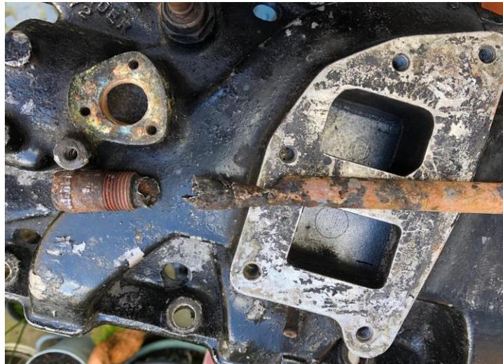
Severely corroded internal **Heater Feed Pipe 90611532**. (Ralph Hardwick)
