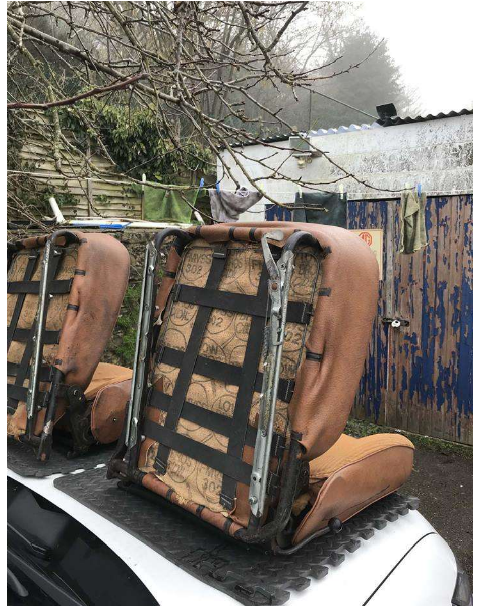
Photo 12 - Even the seats have survived well, no rot, although the webbings seen better days. New webbing is available direct from Brown & Gammons which is great news.
