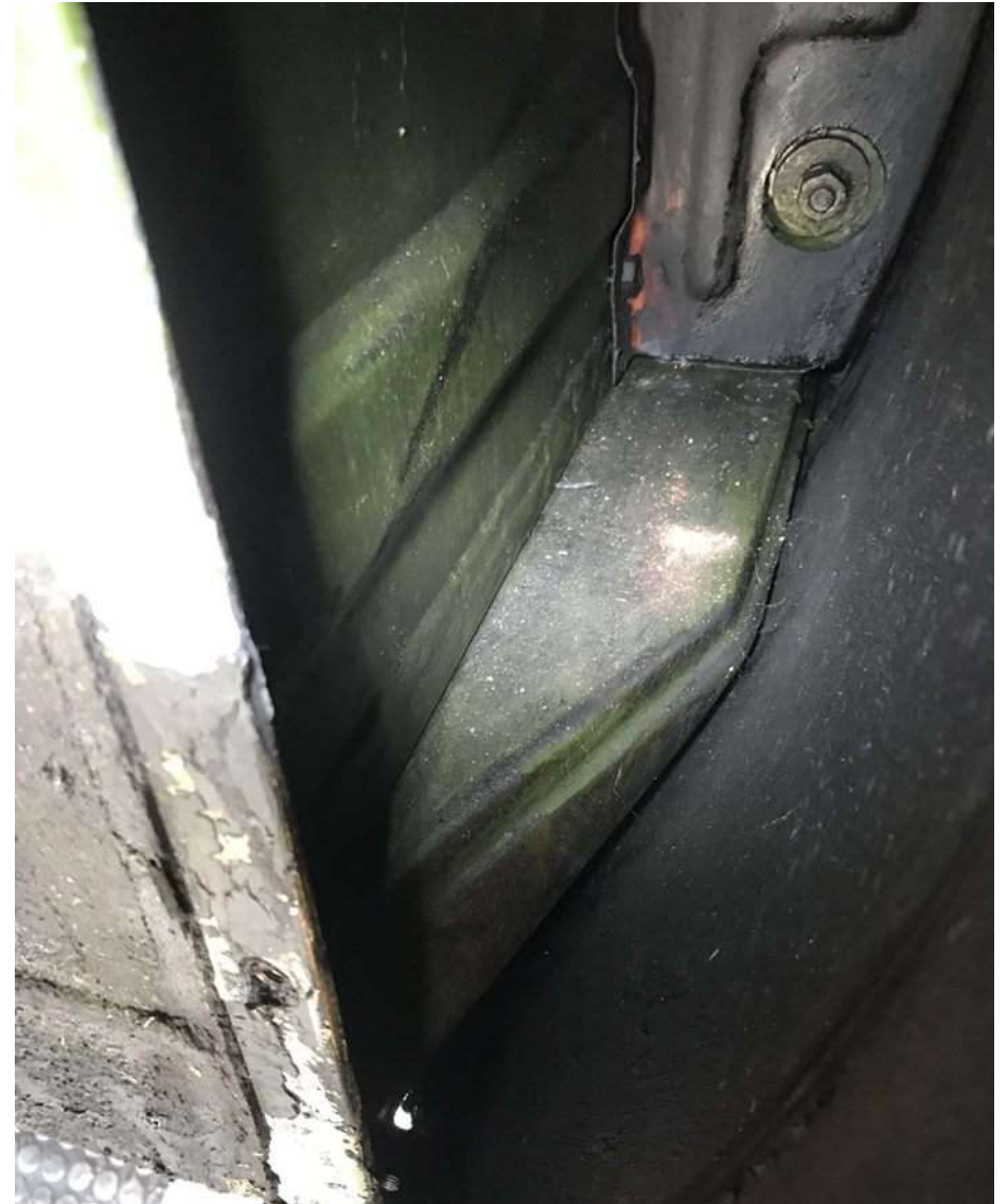
Photo 8 - Removal of the nearside front wing splash guard revealed more solid metal work, great news.
