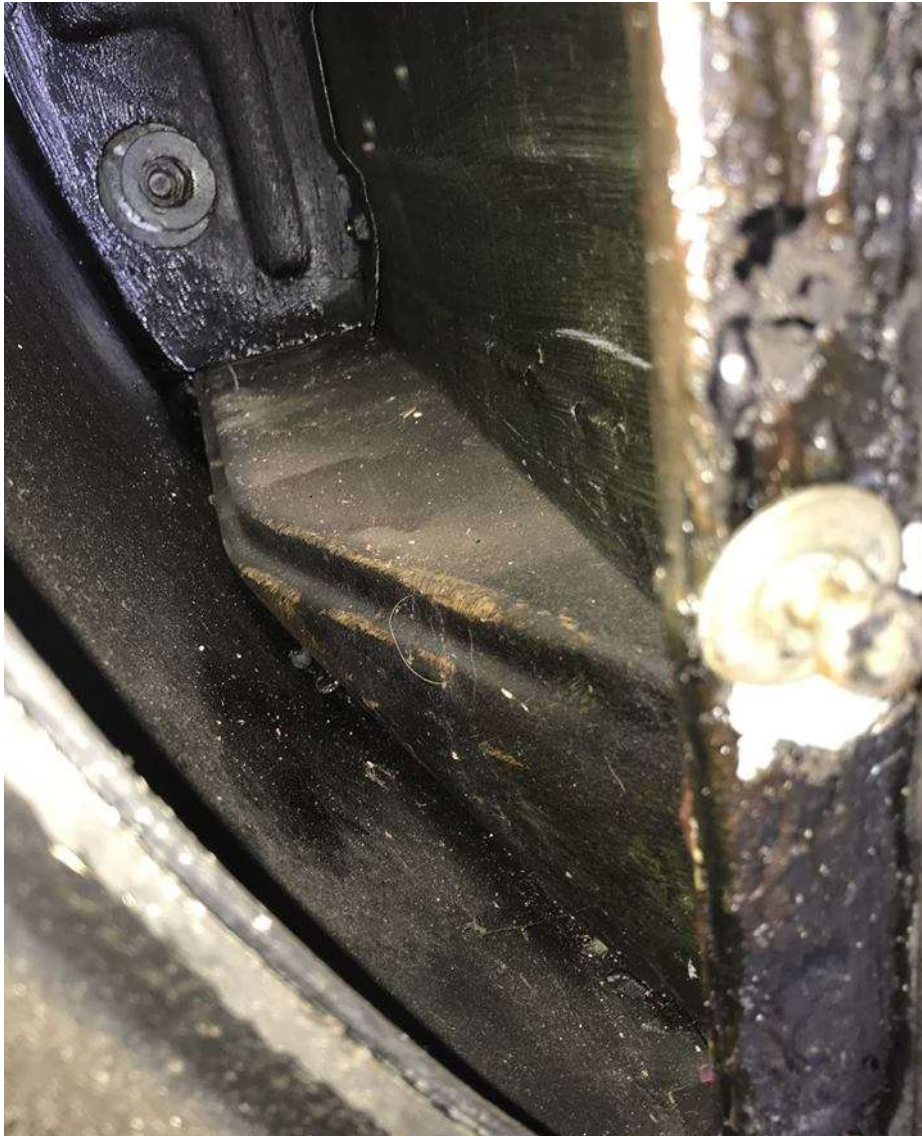
Photo 7 - Crude but thick and heavy front wing splash guards had been fitted. I was keen to remove them and replace with Ashley Hinton stainless steel versions that are pretty much factory spec, in fact better than. Good news awaited behind the splash guards, good solid metalwork soaked in ancient rust proofer.
