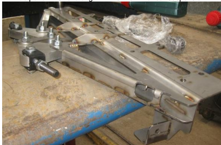
Frontline rear suspension kit showing rocker assembly
