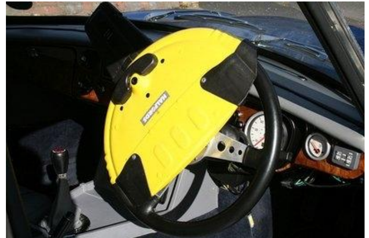
Mike Howlett relies on a steering wheel locking device he bought from Halfords some years ago which is an ideal size for the MGB.
