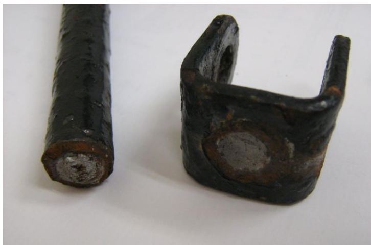
Broken drop link on the front suspension
