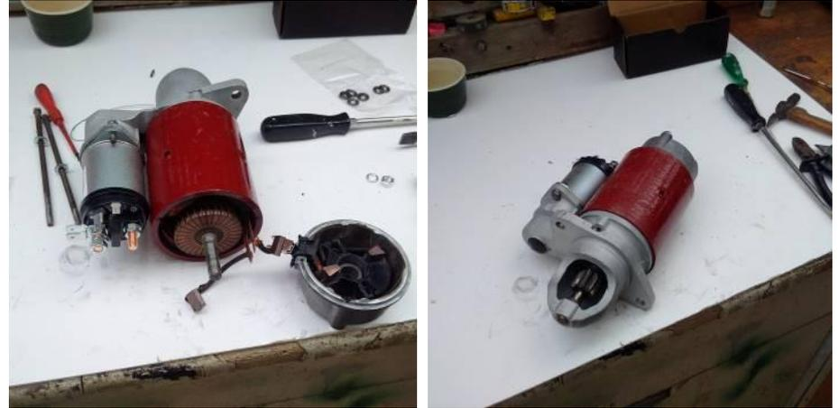
Once the assembly was complete and all screws and bolts tight I tested that it operated correctly. As the starter motor is very powerful with a very high torque capability it was bolted on to the old V8 engine and power applied to the solenoid. The pre select engaged and engine turned over smoothly, when power was removed the cog disengaged and power was removed from the starter windings.
