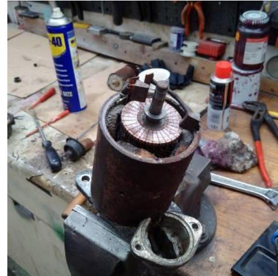
**On with the V8. Today the starter motor.** It was seized solid so before testing the solenoid time to strip and clean the rotor and pre-select assembly. After liberal coating with WD40 the casing screws started to move however the cable connection screws would not budge, used heat and eventually they came undone. Once undone I was able to remove the solenoid fixing bolts and remove it from the starter casing.
