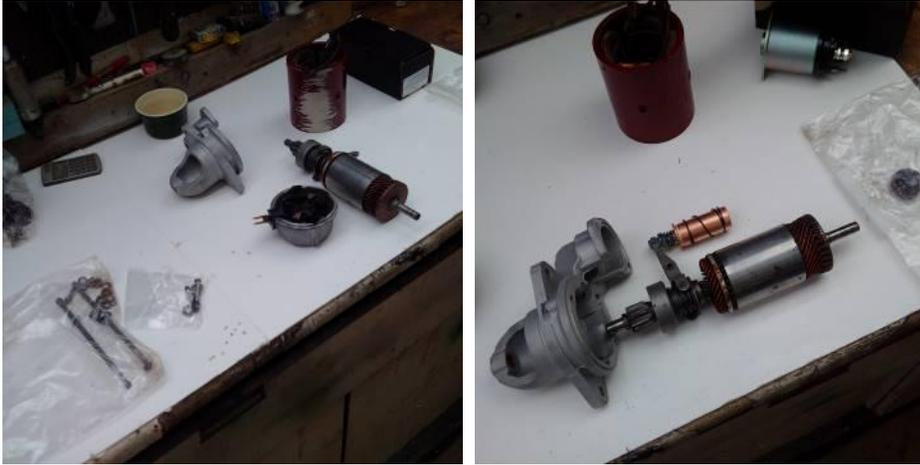
Next the solenoid armature was located on the pre select shaft and the coil was bolted on to the casing. At this stage I tested the solenoid, it operated correctly moving the drive cog to the meshed position and the return spring pushed it back to the disengage position
