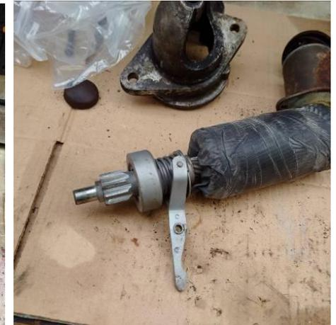
The end cover came off with a little gentle persuasion, the brushes and rotor looked in good condition and the windings checked out showing good continuity and resistance.
