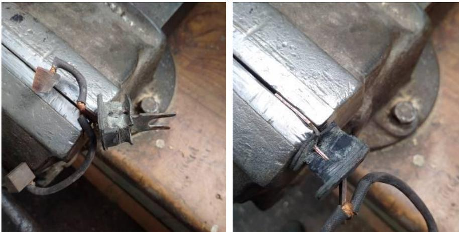
Layer after layer was added over a period of a few days to build it back up to the original size so it seals the casing completely when installed.
