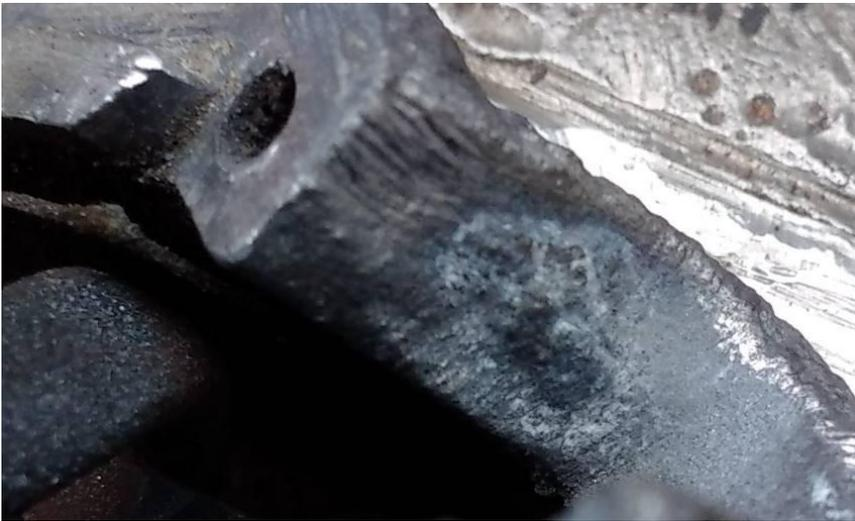
I will build up the rubber insert using Liquid Tape which is an air-dry synthetic rubber coating that can be brushed on. It exhibits excellent moisture, acid, alkaline, abrasion, and dielectric resistance and I have used it before on industrial installations as well as car repairs. Much better than tape.
