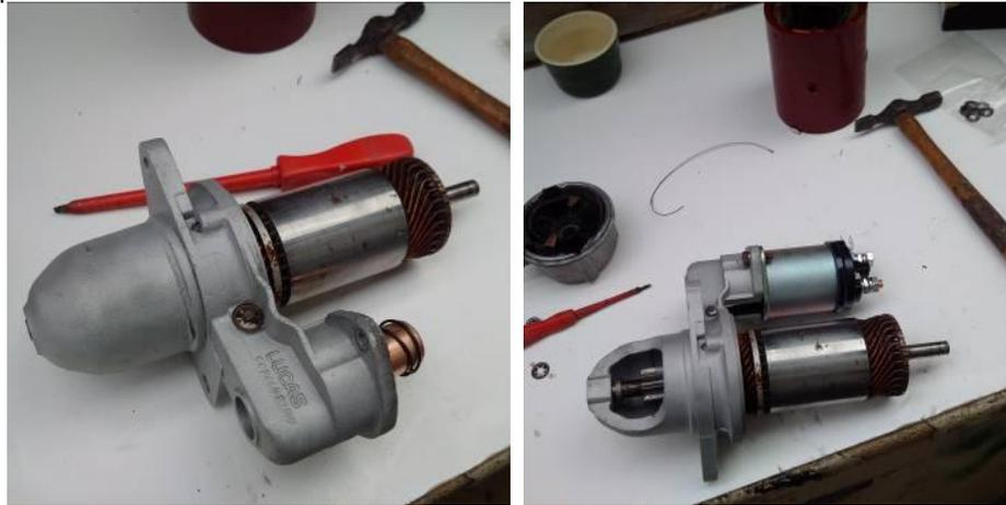
The outer iron case and field windings was then positioned over the armature and located on the peg that is fitted to the casing to ensure that the assembly is correctly orientated.
