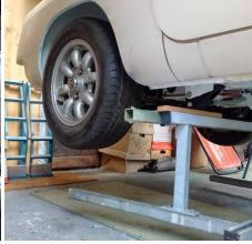
Dropping the back was relatively easy however as the weight transferred to the front the jig decided to slide so the engine hoist was rapidly moved in to position to take the weight.
