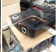
Having drilled the tank I washed all swarf from the internals of the tank using petrol tank cleaner. I pressure tested all soldered joints before installing the pipe to ensure that the pump can self prime. I threaded the take off in to the tank after fitting a fiber washer and a penny washer to the bulkhead fitting internally.
