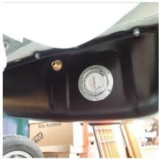
All bolts were smeared with copper ease to protect from corrosion and I will add protective caps once everything is installed under.
