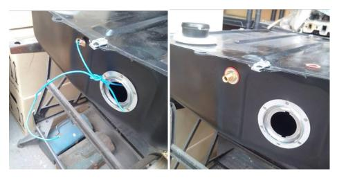
I soldered a compression fitting on to the copper fuel line and for ease made initial bends to the fuel pipe with the tank on the bench using a pipe bender to ensure that the ID is not compromised. I then fitted the fuel sender which is the standard unit without a fuel take off.
