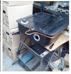
I then fitted strips of self adhesive felt packing to the top of the tank and the tank seal to the fill point to ensure that fumes cannot enter the car. I used the standard fixing kit with fiber washers and fitted blind grommets to all through floor penetrations. When I fit the loom these will be changed to accommodate the loom where required.
