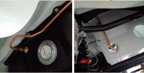
Additional clips will be installed to hold the fuel line once the loom and brake pipes are installed as copper can crack from work hardening normally at fittings due to vibration. The fuel line follows the profile of the body to ensure it clears all moving parts of the rear axle and is clear of the brake lines.
