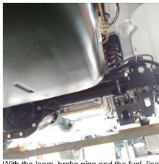
With the loom, brake pipe and the fuel, line installed the next is the battery to starter cable. For this I used red 16 mm tri rated cable flexible cable.
