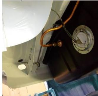
I then fix the loom to the fuel pipe where it crosses above the axle to make sure it cannot foul any moving parts using cable ties. There have been questions as to the "legality" of this with regard to the MOT, however having talked to my MOT garage they told me that it was not a problem as far as they were concerned adding that you cannot fix fuel pipes to the body with cable ties that is a fail as it is not considered "secure" as required by their guidelines.
