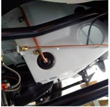
I connected the new brake pipe to the bulkhead fitting where the braded flexible pipe from the back axle terminates. From there I ran it in its rough position under the floor pan to the front of the car.
