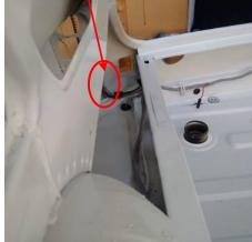
The loom is then threaded through the various body components across the rear of the car to feed the near side rear lights. I reposition the ground point as shown having on this occasion cleaned off the paint and sprayed with WD40m before fixing the cable to ensure a good low resistance electrical connection. This will be tested later when the battery is installed. I also add a "Ground" sticker to make it clear this is an electrical connection and should be maintained on a regular basis.
