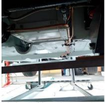
Once the fuel pipe was loosely installed along the length of the car it was run along the side of the off side battery well across the back of the well for protection before entering the well which is now the petrol pump well and connected to the red top pump outlet via a flexible braded petrol pipe.
