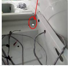
The cable is clipped to the underside of the boot floor support to the rear of the car. Grommets are used everywhere to protect the cables and to prevent ingress of water or
