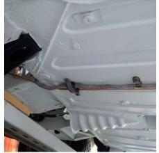
Once the brake pipe was loosely positioned the fuel pipe was installed from the fuel pump forward to the engine compartment.
