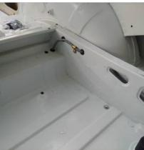
I ran the fuel sender cable through what would be a spring support point to the chassis which are now unused as the 5 link suspension does not use the rear supports. It then runs along the chassis leg held with two clips. Once the installation is complete I will add a protective cover to protect the connections to the sender
