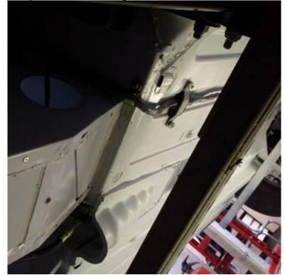
I then loosely installed the front loom. The reason for this was to ensure that the two looms, front and rear meet at the correct location.
