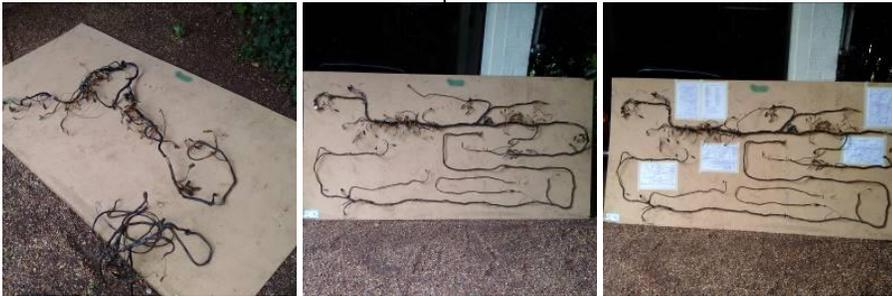
To do this I mounted the loom on a board as shown above and worked from one end to the other initially cleaning the cables then stripping the tape a section at a time.
