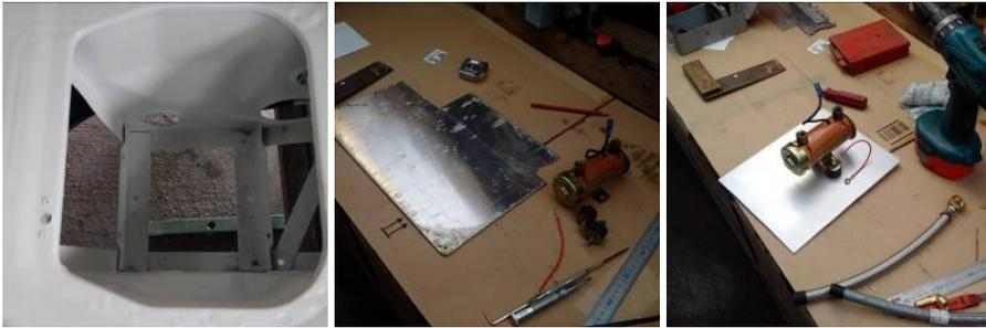
The pump backplate was made from 1/8" aluminum for rigidity where as the bottom plates were made from 1/16" mild steel. The pump backplate was fitted using studs for easy removal and rubber sealer to prevent the ingress of water. The bottom plates were pop riveted in position with Tiger seal between the chassis frame and the plates.
