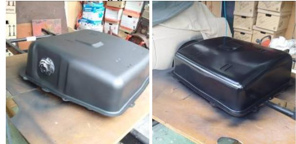
I do not like the position of the fuel pump on the V8 and as I intend to install a 12 V battery in the spare wheel well I decided to modify one of the 6 volt battery bays to accommodate the pump. The main advantage is to keep the fuel pump dry and easy access to the pump filter from the inside of the car.
