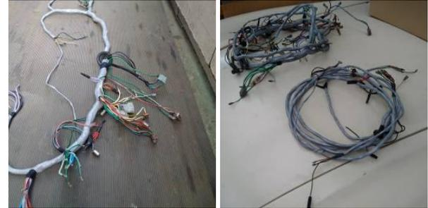
Once the work on the loom was complete a continuity check was carried out and all tested out correctly.
