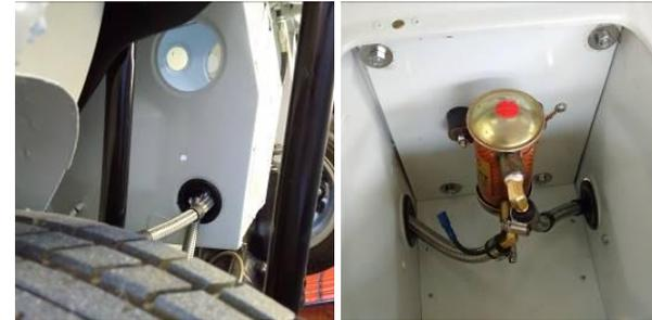
Flexible ethanol resistant ss covered fuel pipes will be used to connect to the 3/8" copper fuel feed system.
