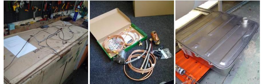
I had a red top fuel pump from a previous rebuild of my MGB GT and a fuel filter which I intend to use on the V8. The fuel tank was cleaned and primed with a suitable primer for the galvanized tank then sprayed with stone chip before finishing with semi gloss black paint to match the rest of the running gear.
