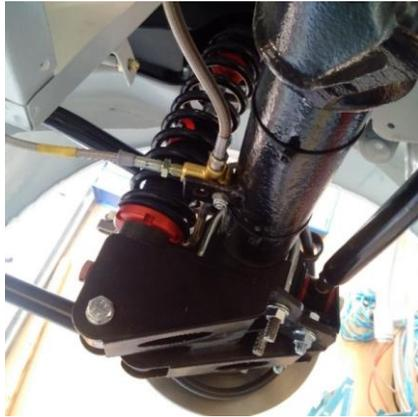
Once the hydraulic lines were installed the hand brake cables were next. These required a bracket to be installed adjacent to the transmission tunnel.
