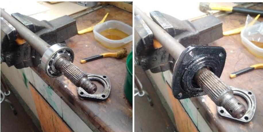
Two brake caliper mounting plates were then installed that replace the backplate.
