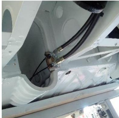
Again although not included in the kit I added P clips to ensure that the brake cable could not be snagged by anything while driving. These were a loose fit to allow the cable to float as the hand brake is operated.
