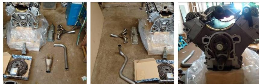
I put the old engine on the engine stand and removed all the parts needed ready for cleaning, painting where necessary and assembling on to the new strip engine.
