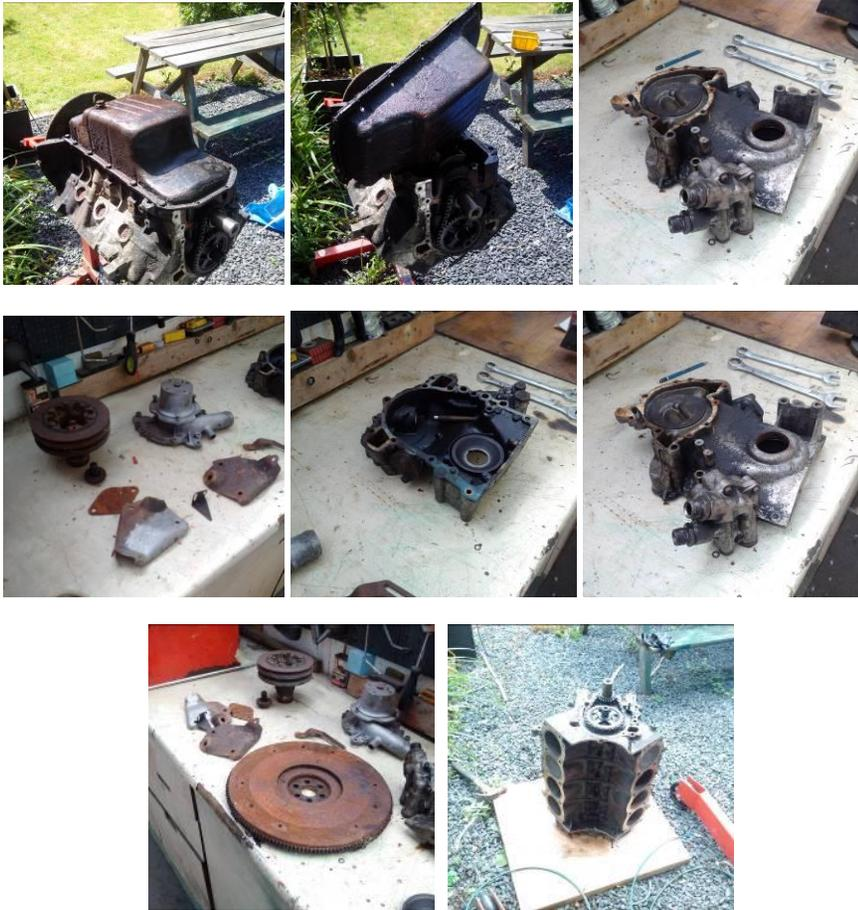
With all the parts removed the old engine will be cleaned and the heads and valve gear replaced. The engine was about the only part of the car that ran correctly when I bought it so I hope it can be used by someone else in an MG V8.
