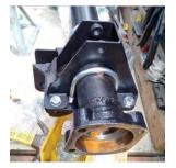
Once the lower axle brackets were fixed the upper brackets were positioned on the axle and the U bolts installed through the upper and lower brackets. Tightening of the U bolt nuts was done sequentially ensuring that the threaded legs were all of equal length. The U bolts were tightened to 30lb ft torque.
