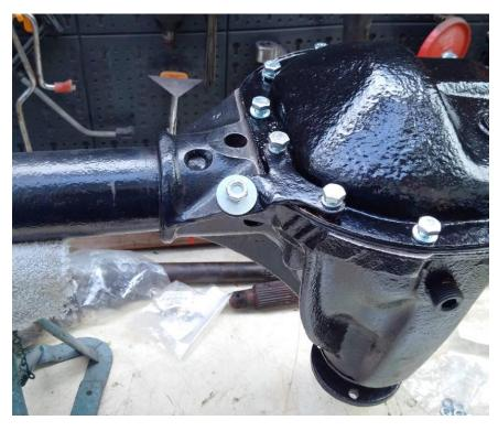
**New oil drain and fill plugs** were I installed coated with copper ease to prevent them seizing in the future. I also installed a **LR brass axle breather** on the axle in place of the plastic unit.
