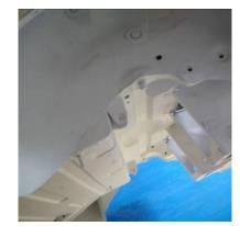
Once this coat was dry, **stone chip was sprayed on the wheel arches** and areas likely to be damaged by stones thrown up by the rear wheels. The stone chip paint is available in two versions, both black, one has wax included and is therefore not suitable for over painting. I chose the type that can be overpainted as I wanted the underside to be Glacier White.
