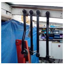
The **5 link suspension system** was then reinstalled on the shell, through body penetrations for fixing bracket fixings were sealed using a polyurethane adhesive sealant to prevent water ingress.
