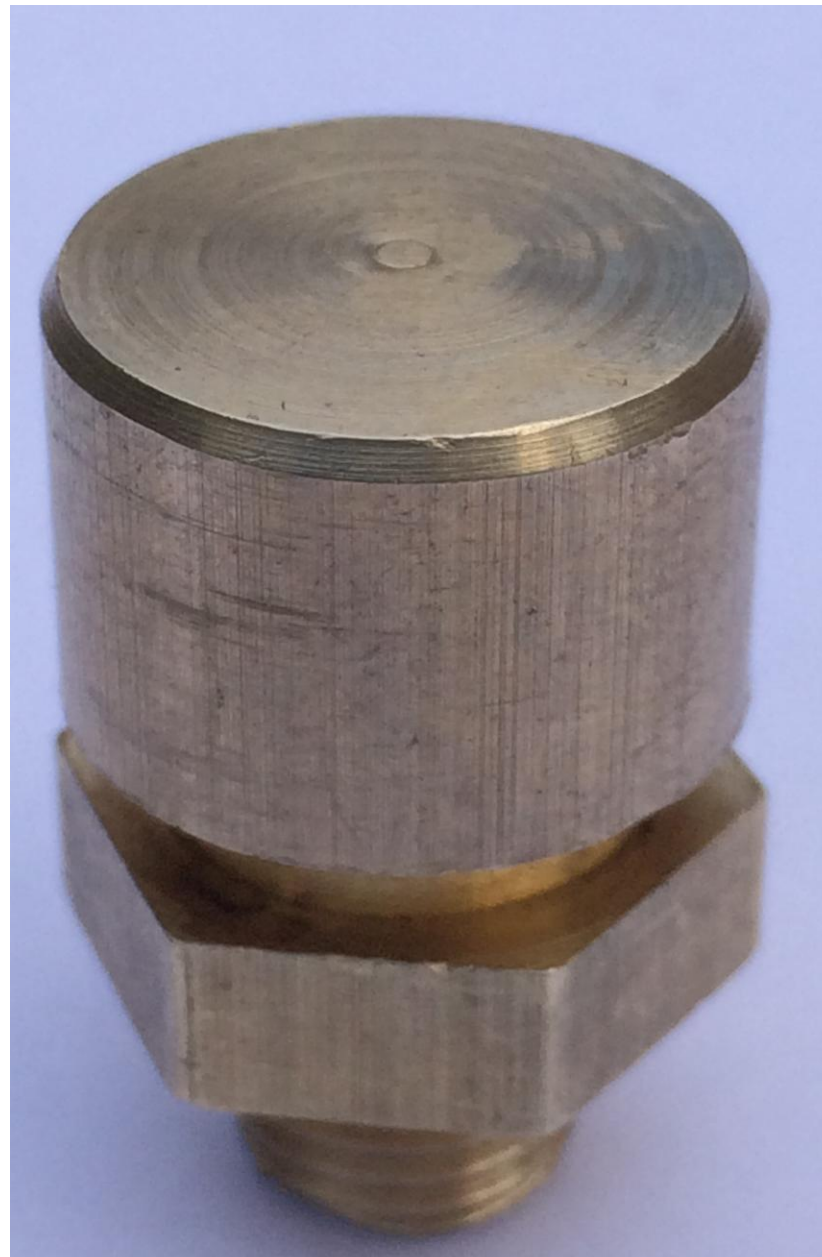
Brass breather valve as fitted to Land Rover back axles – you can see brass part fitted to an RV8 back axle. More
