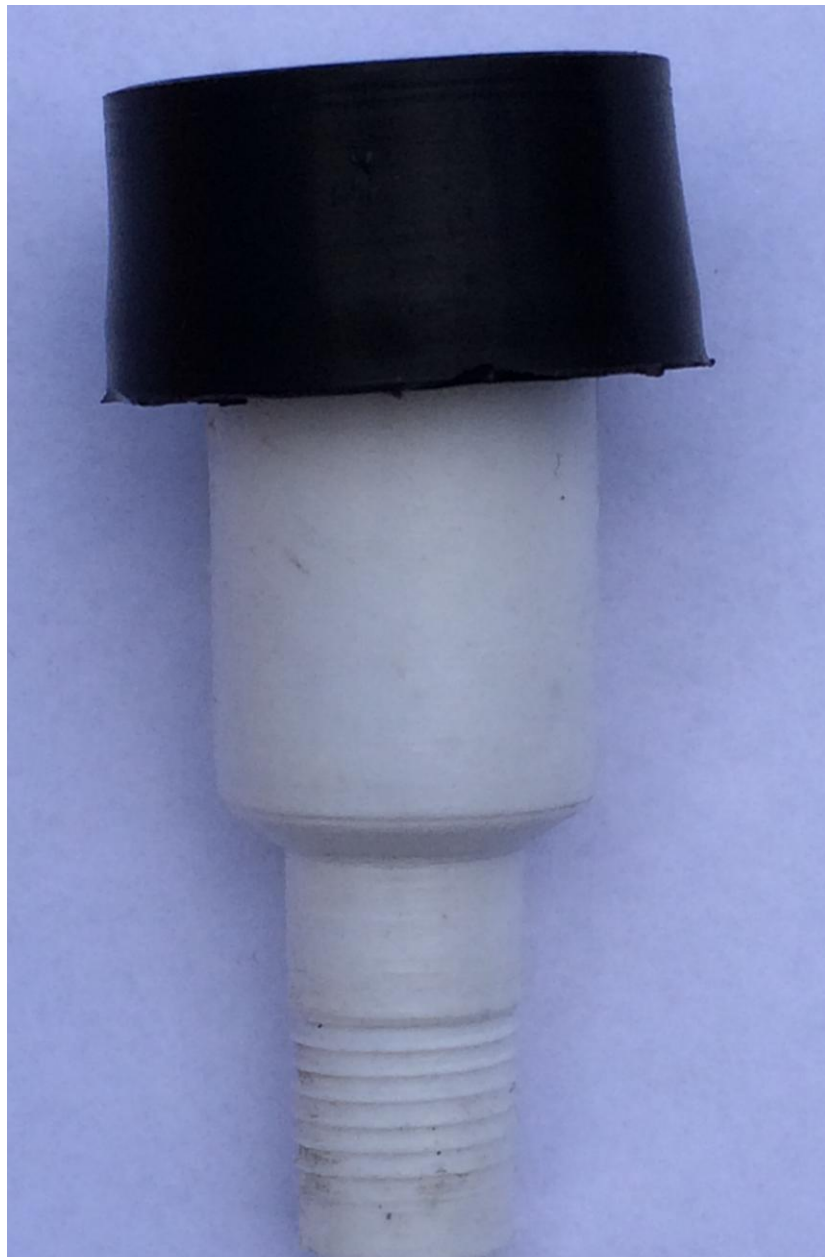
Replacement plastic breather valve the quality of which on inspection was not very good. See RV8NOTE413
