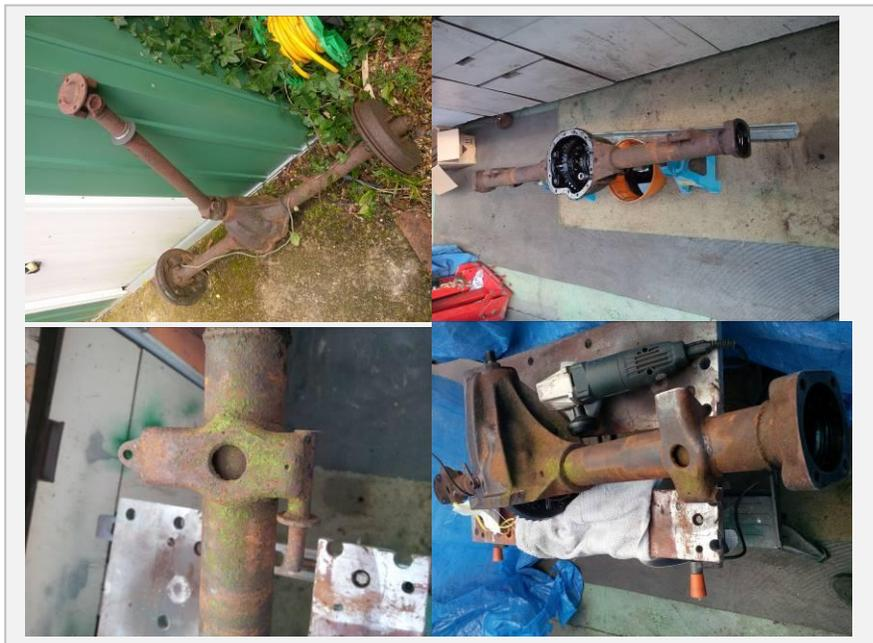
After grinding off the front tab and the rebound strap mounting point I degreased the axle and painted it with rust prevention paint. All other components were degreased and where required painted.
