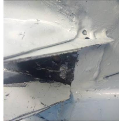
After cutting the web sides I drilled the spot welds out so that the new spring hanger mounting bracket will sit flush with the spring hanger.
