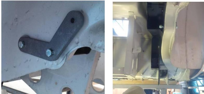
Once installed I found that the hole in the sub-frame did not line up with the hole in the spring hanger.
