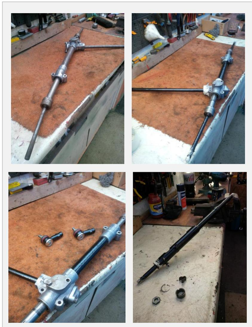
Once all the steering components were restored I installed them in the body shell having sprayed the front section of the cockpit. Care was taken aligning the steering rack and the column. Spacers were installed under the rack to cross member mounting points as required to achieve the required alignment.
