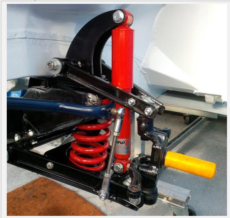
Having completed the suspension I looked at the brakes with the intention of restoring the old ones however the disks were badly pitted and one of the calipers had a crack across the mounting point so were discarded replacement V8 calipers are hard to come by so an alternative. On my MGB GT I have a Wilwood twin pot system with ventilated disks and I decided that a twin pot system was the way to go with the V8 especially as the engine I intend to install is a 4.0 L. I looked at
