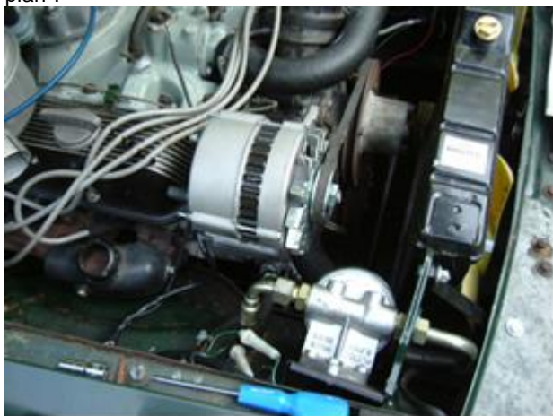
Upated alternator with the cooling fans at 2,600rpm.
