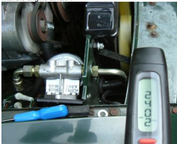
Original AC Delco alternator with the cooling fans at 2,402rpm.
