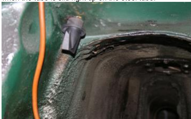
The new drain tube in place - the brown tube is the petrol feed pipe.
