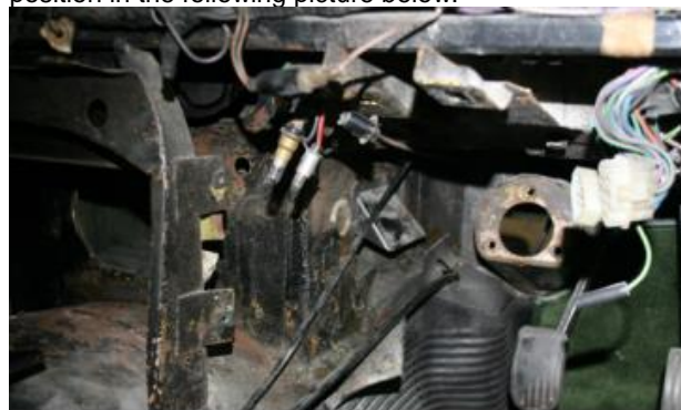
Centre console removed - note the white plastic plug just to left of footwell heater outlet.
