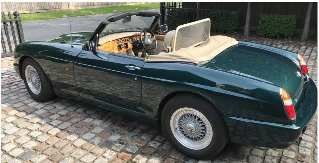
Attractive 15 inch spoked, machine polished and lacquered alloy wheel by Alloy Wheels International was fitted to the RV8 as standard. The "rivets" are dummies (supplied by Zender) as the wheels are single piece and not split rimmed (like the contemporary Compomotive wheel) as they might appear.
