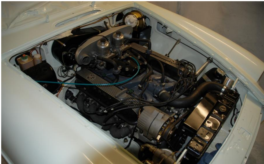
A very neat installation in an early chrome bumper MGBGTV8
