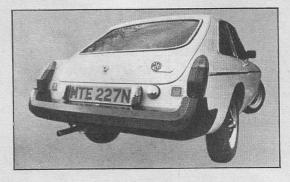
Bayflex system. Meeting the US Federal legislation re 5 mph collisions Bayflex was found to be the only material that meets all requirements—is flexible, highly resilient and satisfies the aesthetic demands made on an exterior body part. Bayflex bumpers are the result of the most advanced research and testing and provide the lastword in vehicle protection. It's yet one more example of how Bayer technology is helping to build better cars and make the roads a safer place.
